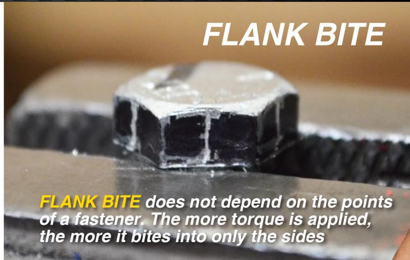
**FLANK BITE** does not depend on the points of a fastener. The more torque is applied, the more it bites into only the sides
