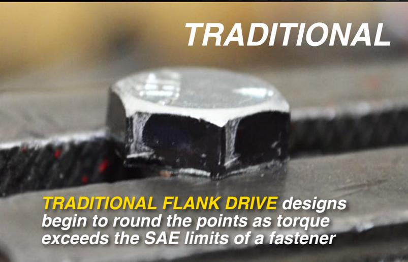
**TRADITIONAL FLANK DRIVE** designs begin to round the points as torque exceeds the SAE limits of a fastener
